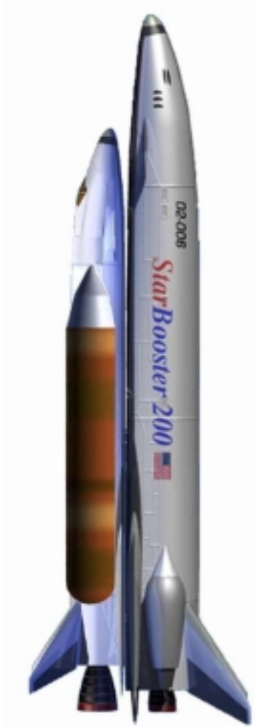
Figure 5 StarBooster200 TM & StarBird I TM Launch Configuration – Parallel Burn
